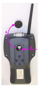
• Press the reset button with a pencil (B), if the device has no external power supply connected, it will switch off.
